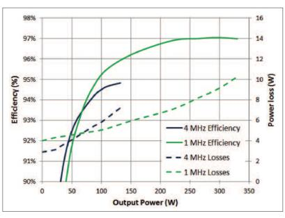
Figure 3: Efficiency results for EPC9006 and EPC9002 demonstration boards in ET application operating at 45 V input and 22 V output voltage
