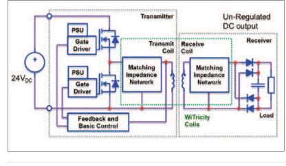
Figure 1: Schematic block diagram of the evaluated wireless energy system
