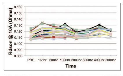
Figure 3: Source-drain resistance of 600 V rated cascode switch for a population of representative cascoded GaN-on-Si based HEMT devices with  $W_s = 120$  mm, under a drain bias of 480 V and 0 V gate bias for 5000 hrs at 150°C
