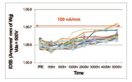
Figure 4: Source to drain leakage current measured with 500 V drain bias and 0 V gate bias of 600 V rated cascode switch for a population of representative cascaded GaN-on-Si based HEMT devices with  $W_s = 120 \text{ mm}$ , under a drain bias of 480 V and 0 V gate bias for 5000 hrs at 150°C
