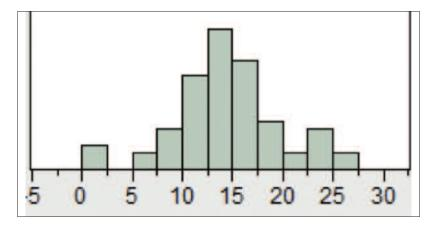
Figure 1: Measured distribution of final wafer bow for over 20 multi-wafer process runs producing more than 60 crack free 2.25 µm thick AIGaN alloys based hetero-epitaxy on 200 mm standard thickness (725 µm) Silicon substrate
