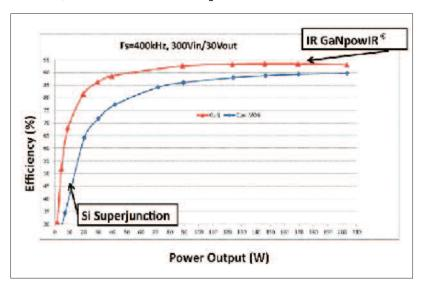
Figure 5: Measured conversion efficiency for a resonant LLC converter with 300 V input and 30 V output voltage operating at 400 kHz, using either IR's GaNpowIR<sup>®</sup> based devices on both the primary (600 V rated) and secondary side (100 V rated) of the transformer (with synchronous secondary side rectification) or state-of-the-art Silicon alternatives
