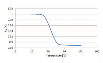
Figure 3: Thermal resistance versus heatsink temperature
