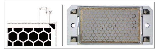
Figure 2: Dimension and pattern after screen-printing
