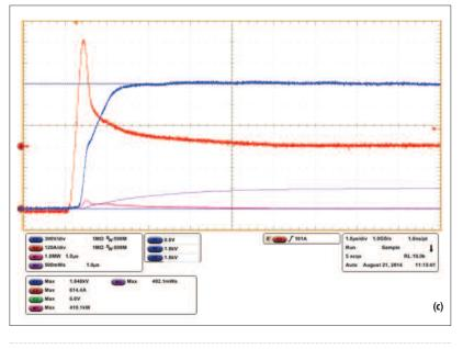
Figure 6: Switching waveforms of FF450R33TE3 for turn-on (a), turn-off (b) and recovery (c) at nominal conditions 1800 V /  $125^{\circ}$ C
