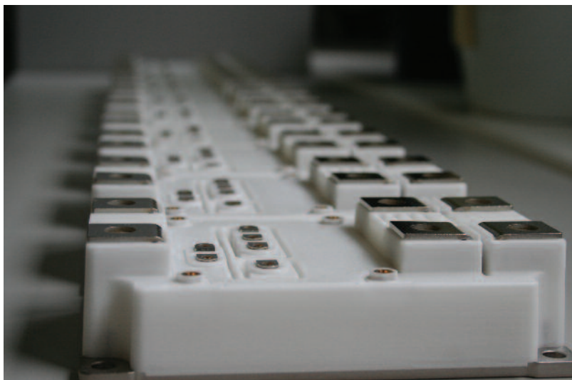
Figure 1: ABB's low inductive LinPak IGBT module for reliable high-power converters
