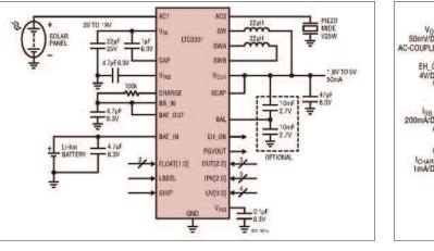
Figure 3: LTC3331 solar energy harvesting application
