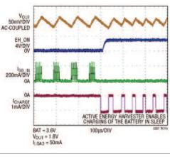
Figure 4: Battery charging process
