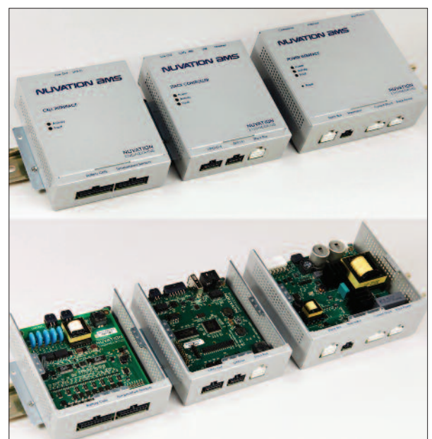
Figure 2: The three major subsystems of the Nuvation BMS - cell interface, stack controller, power interface - comprise a modular, hierarchical design which results in scalability, robustness, and reliability across a wide range of power levels as shown in the block diagram (above) and physical realization (right)
