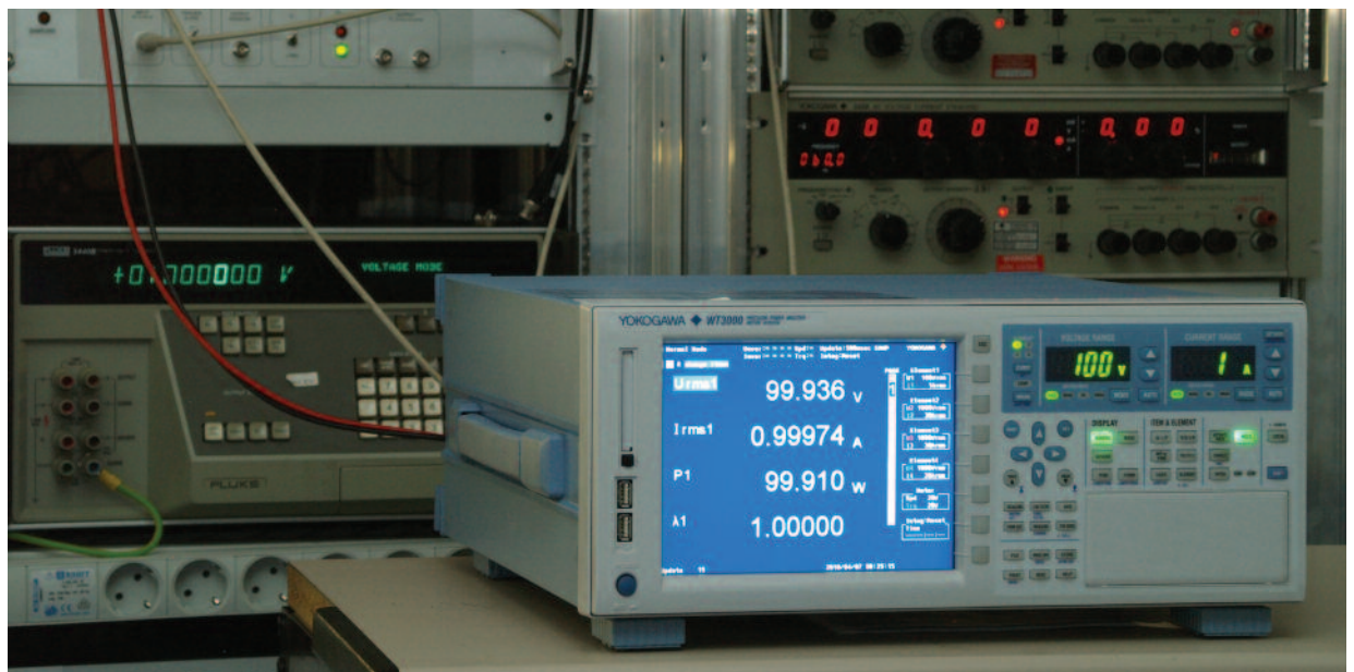
Figure 3: The WT3000 precision power analyzer
