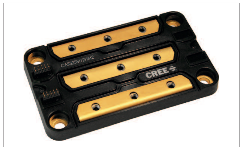
Figure 1: The CAS325M12HM2 All-SiC power module with a 5.5 nH power-loop inductance uses a high-speed internal signal distribution board for equalized die performance
