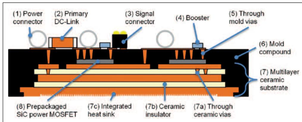
Figure 1: Vertical layer stack of the molded power module with SMD assembly
