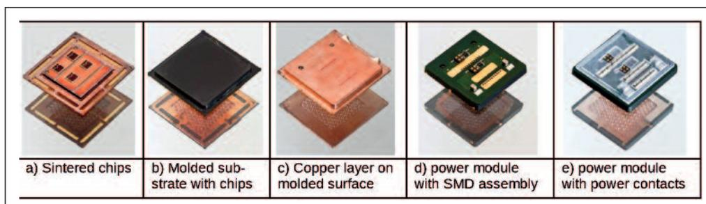
Figure 4: Manufacturing steps of the molded power module
