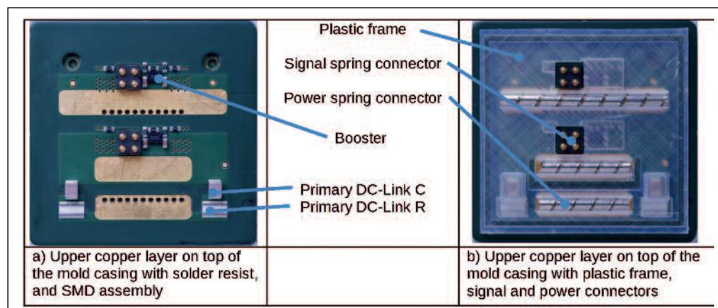
Figure 2: Top view of the molded power module
