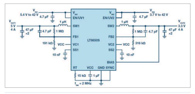
Figure 2: Simplified LT8650S schematic delivering 5 V at 4 A and 3.3 V at 4 A outputs, at 2 MHz
