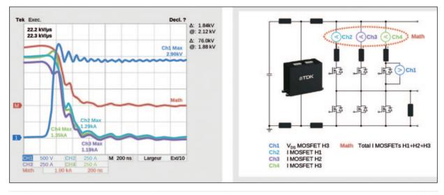
Figure 5: The new HF film capacitor series features extremely low voltage overshoot and ringing
