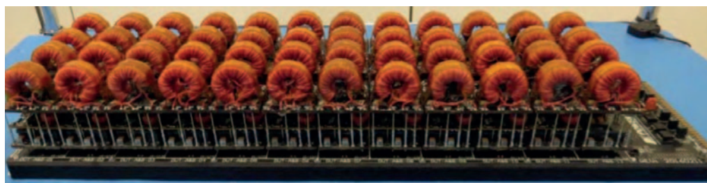
Figure 3: DOPL stress-test board used for PowiGaN InnoSwitch3 device qualification testing
