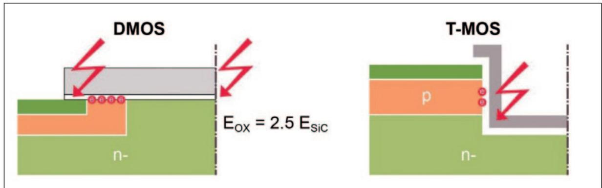
**Figure 2: Typical structure of a planar MOSFET (half-cell) revealing two sensitive areas with respect to oxide field stress (left) and typical structure of a trench MOSFET (half-cell), critical issue is the oxide field stress at the trench's corners**
