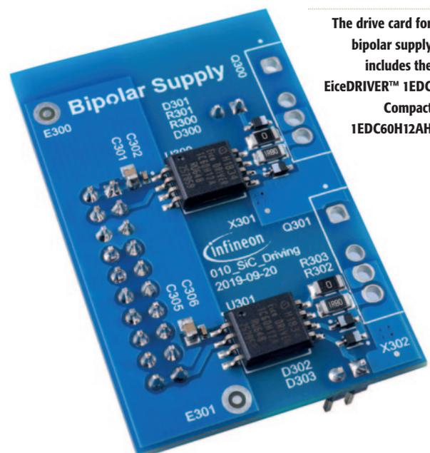
The drive card for bipolar supply includes the EiceDRIVER™ 1EDC Compact 1EDC60H12AH
