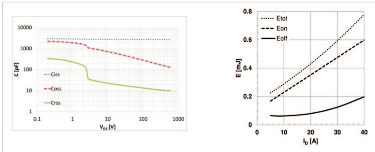
**Figure 4: Typical device capacitance vs. drain-source voltage for a 45 mΩ CoolSiC (left) and related switching energies (right) as a function of drain current (for  $V_{GS} = 15/-5$  V,  $R_{Gext} = 4.5$  Ω,  $V_{DS} = 800$  V,  $T_{vj} = 175^{\circ}\text{C}$ )**
