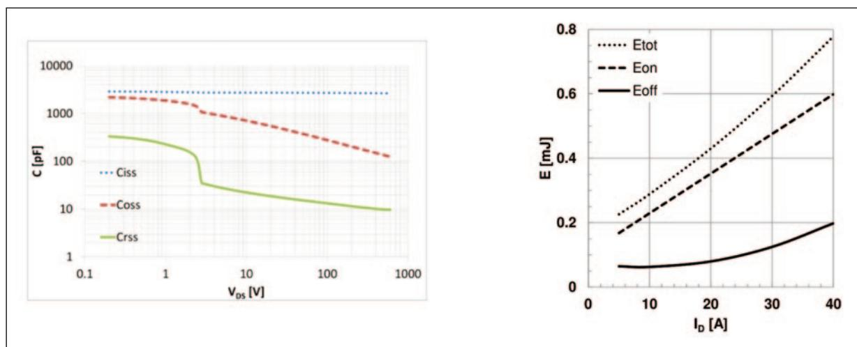
**Figure 4:** Typical device capacitance vs. drain-source voltage for a 45 mΩ CoolSiC (left) and related switching energies (right) as a function of drain current (for  $V_{GS} = 15\text{--}5\text{ V}$ ,  $R_{ext} = 4.5\text{ }\Omega$ ,  $V_{DS} = 800\text{ V}$ ,  $T_j = 175^\circ\text{C}$ )
