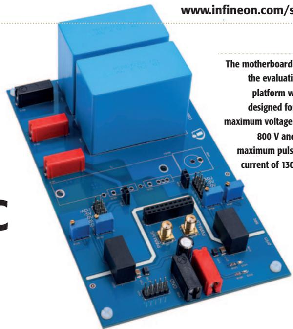
The motherboard of the evaluation platform was designed for a maximum voltage of 800 V and a maximum pulsed current of 130 A
