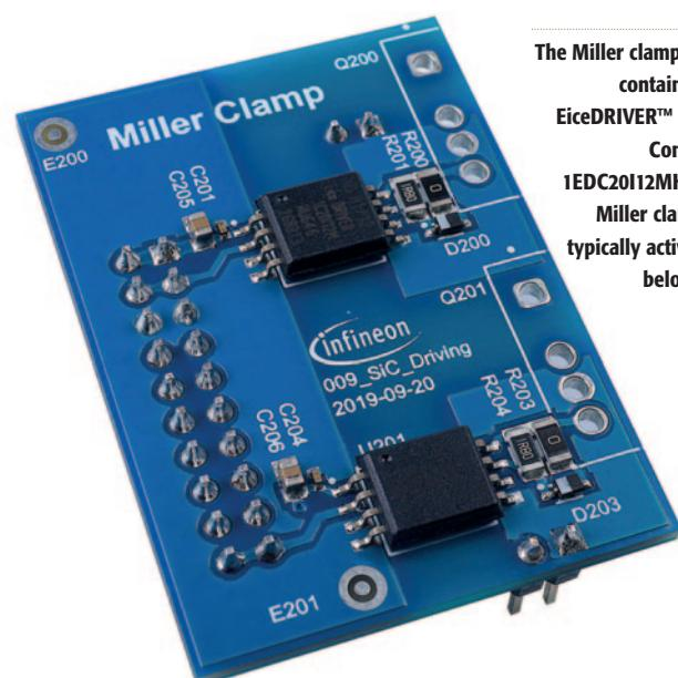
The Miller clamp card contains the EiceDRIVER™ 1EDC Compact 1EDC20I12MH, the Miller clamp is typically activated below 2V
