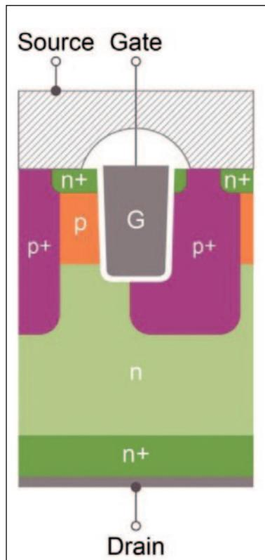
**Figure 3: Sketch of the CoolSiC MOSFET cell structure**
