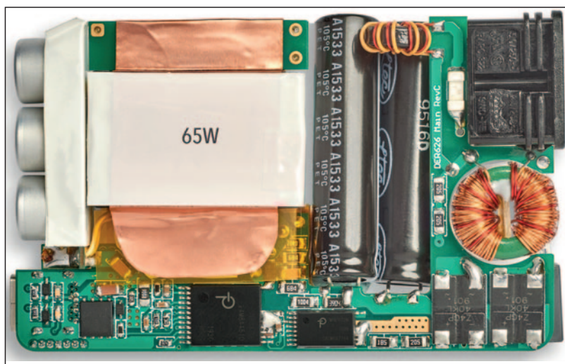
Figure 6: With MinE-Cap IC, InnoSwitch3-Pro IC and low-profile planar magnetics, a form factor of 82 mm x 51 mm x 12 mm for the 65 W design was realized
