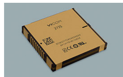
Figure 5: The DCM3735 is a non-isolated, regulated DC-DC converter with an input range of 35-58V. It offers constant current operation for battery charging, comes in a compact package (36.6 x 35.4 x 7.4mm) and can be used in array.
