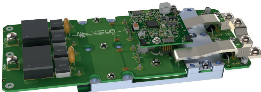
Figure 4: This 4kW DC-DC converter uses 2 Vicor BCM6135 and 2 DCM3735 (located on the underside of the board) to convert 800V power to 12V power in a package that weighs 0.08 kg and in a volume of only 0.8575 L. This can be configured into 2 redundant power supplies of 2 kW each, or paralleled with another unit to create a redundant 4 kW power supply.
