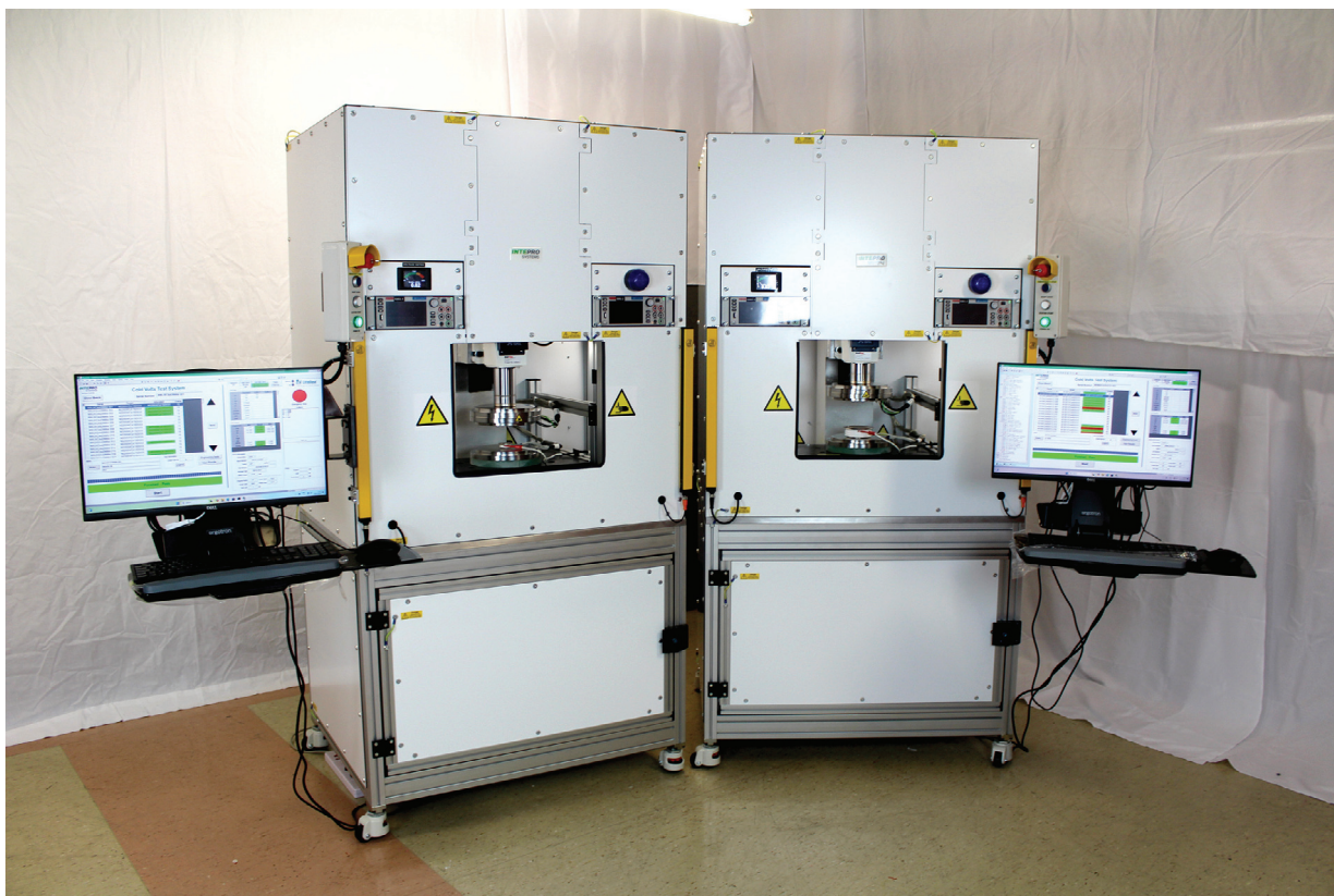
Automated Test Equipment (ATE) systems serve the critical purpose of ensuring that electronic devices operate according to specifications in the field.
