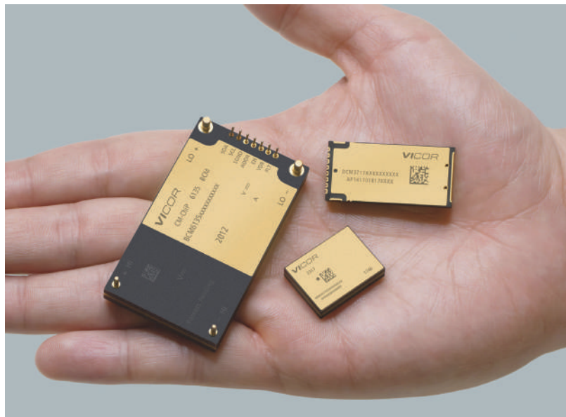
Figure 5: Vicor high-performance power modules provide kilowatts of power in a small space.
