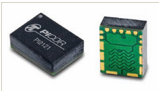
Figure 1: Full function active ORing solution of 5 x 7 x 2mm thermally enhanced LGA
