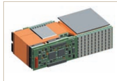
Figure 4: 3D CAD drawing of 10kW/litre, 5kW DC/DC converter
