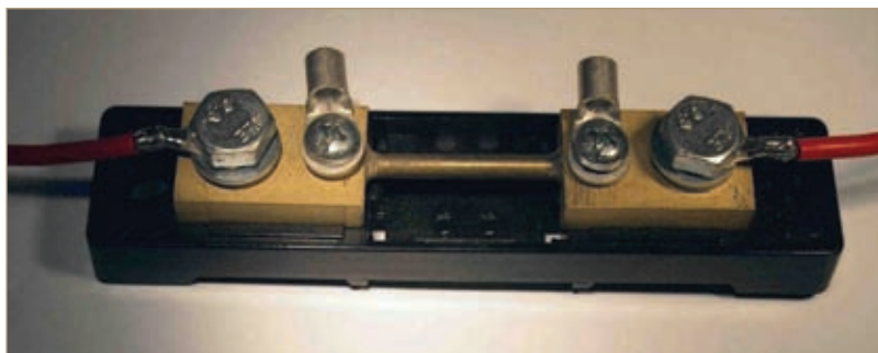
Figure 2: Shunt with four terminals
