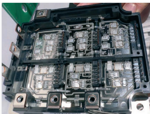
Figure 1: Opened three-level IGBT module
