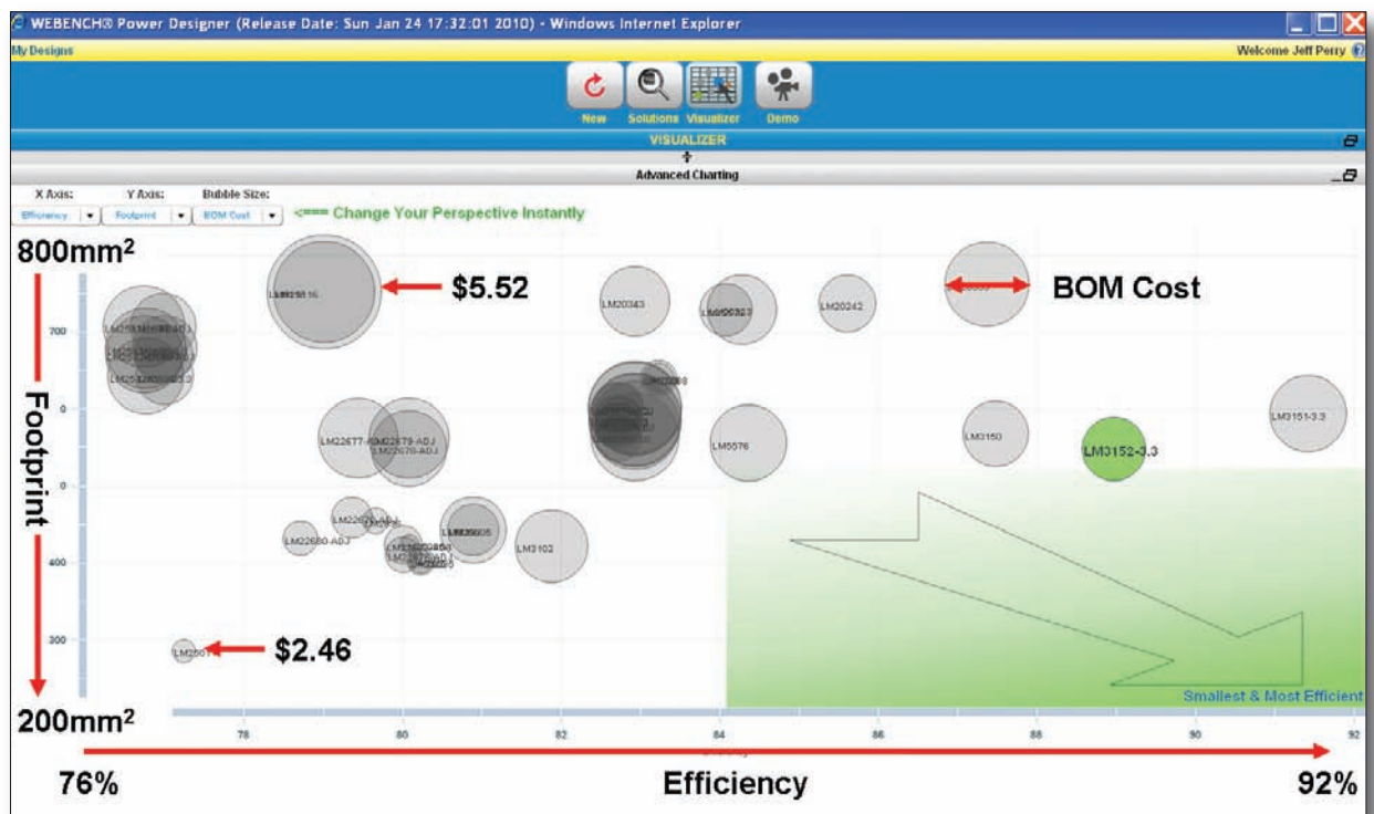
Figure 1: Graph of 50 different power supply solutions for a given set of inputs showing trade-offs between footprint, efficiency and BOM cost
