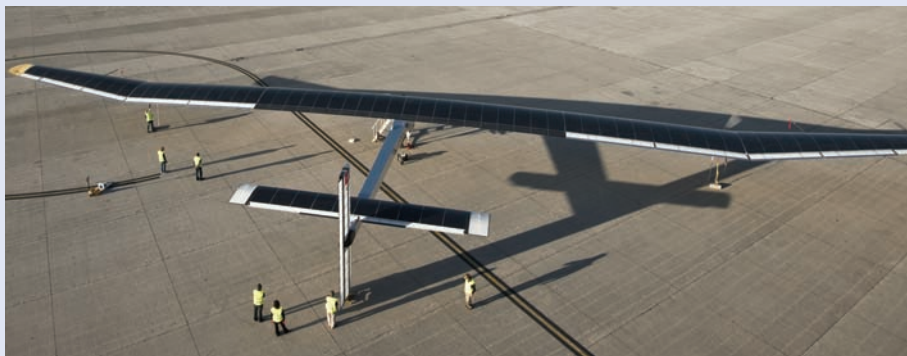
HB-SIA has a wingspan of 63.4m, 12,000 solar cells are integrated into the wing to supply four electric motors
