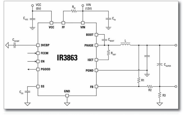
Figure 1: Proposed super capacitor charger circuit
