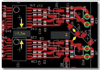
Figure 5: Two adjacent IGBT drivers on the driver board and the creepage distance
