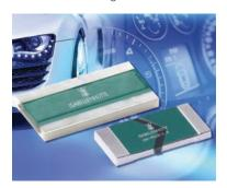
temperatures up to 125°C. Consequently, resistors used in LED technology have to be very small, perform extremely well, be extraordinarily robust, highly stable and have a small tolerance. Isabellenhütte's VMK resistors have the required specifications: 1 W permanent power up to 110°C terminal temperature; constant current up to 10 A (10 m $\Omega$ ); small size (1206; 3.2
