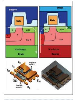
Cross section of Drain Down (left) and Source Down (right) NexFET Power MOSFETs and Power Block structure (bottom) Source: TI
