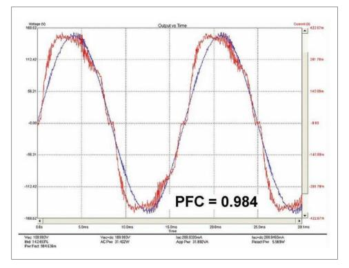
Active power factor correction provides smooth input current waveforms (red) and power factor of 0.984 in this setup
