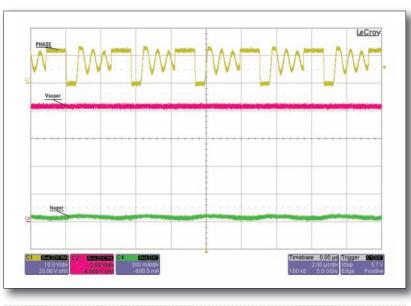
Figure 4: Typical converter switch node waveform during the final charging stage
