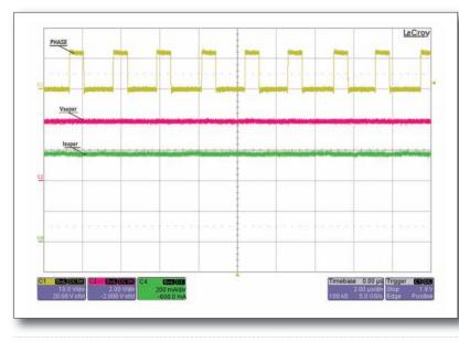
Figure 3: Typical converter switch node waveform during the initial charging stage
