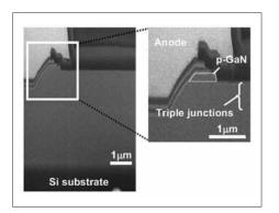
Cross sectional Scanning Electron Micrograph image of the Multi-Junction Diode Source: Panasonic
