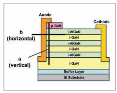
Cross section of GaN-based Multi-Junction Diode with reverse leakage current using p-type barrier controlling layer Source: Panasonic
