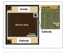
Chip photograph of the Multi-Junction Diode
