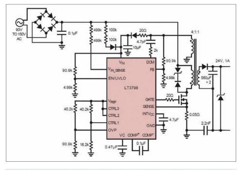
Block diagram of the isolated flyback controller LT3798 with single stage active power factor correction
