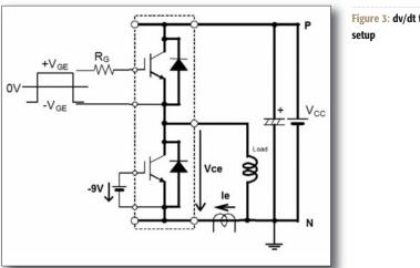
the turn-on energy has been modified to keep the device under test "non floating". This modification of the test setup (Figure 3) allows keeping the oscilloscope on a stable and non floating potential.
