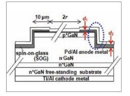
Cross section of Hitachi's GaN p-n diode with mesa-fieldplate edge termination. The domain of the dotted ellipse is shown in the next image on the left Source: Hitachi
