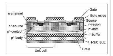
Cross section of Panasonic's SiC DioMOS with the thin channel layer Source: Panasonic
