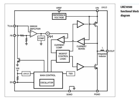
the PFET switch on-time. The circuit generates a duty-cycle modulated rectangular signal. The rectangular signal is averaged using a low pass filter formed by the integrated inductor and an output capacitor. The output voltage is equal to the average of the duty-cycle modulated rectangular signal.
