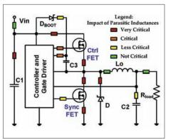
Schematic of synchronous buck converter with parasitic components Source: TI
