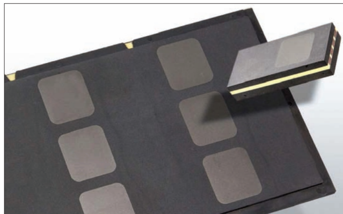
Vicor's new ChiP power components are sawn out of scalable magnetic panels
