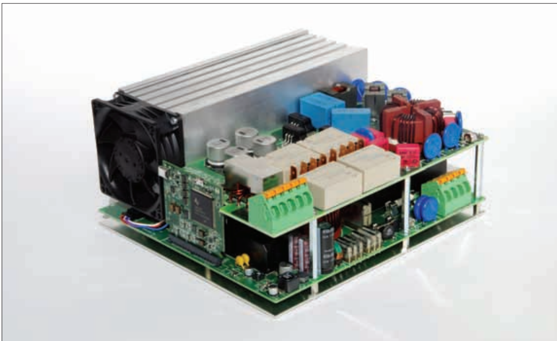
Fraunhofer ISE developed a three-phase 10 kW UPS inverter with a volume of just five liters and an efficiency of 98.7 percent
