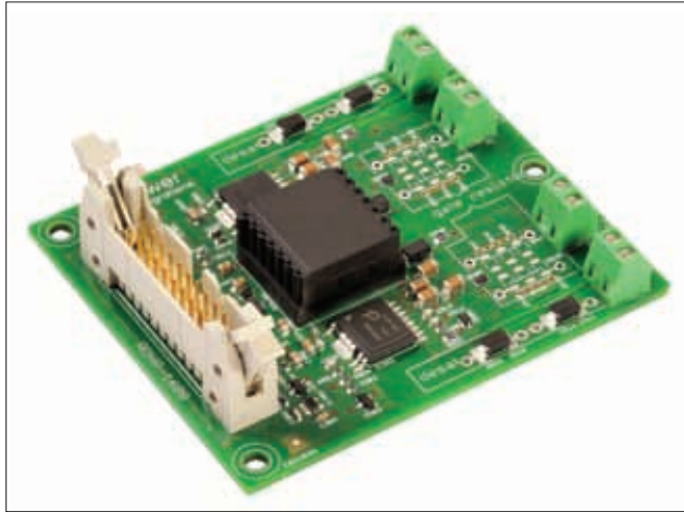
Figure 2. A design using two SID1182K devices and a single isolated power supply
