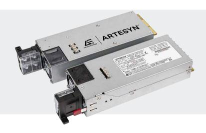
Advanced Energy's Artesyn CSU2000ADC is housed in the industry standard  $1U \times 73.5 \times 185$  mm form factor featuring -48Vdc input voltage. This DC/DC power supply belongs to the CRPS family of products, and matches the mechanical form and fit of Advanced Energy's AC/DC power supplies. The common form, fit, and function for all products in the family provides a path for power capacity flexibility, future-proofing your system designs.
