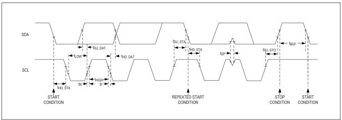
Figure 22. Detailed I<sup>2</sup>C Timing Diagram
