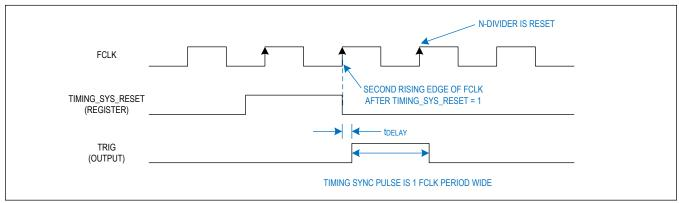
Figure 2. Timing System Synchronization with MAX30009 as a Master
