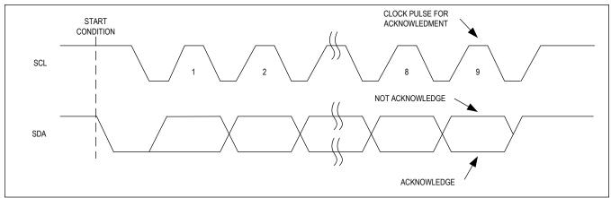
Figure 24. I<sup>2</sup>C Acknowledge Bit
