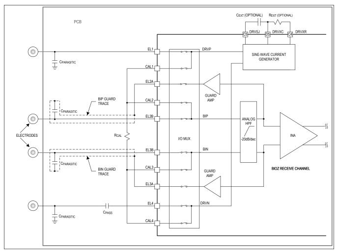
Figure 17. Calibration Port Connections
