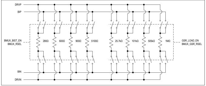
Figure 13. Programmable Resistor Load
