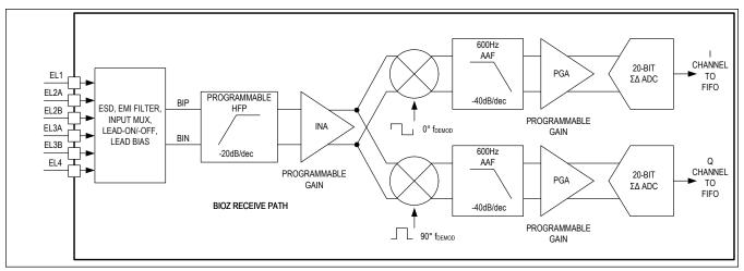
Figure 10. BioZ Receive Channel
