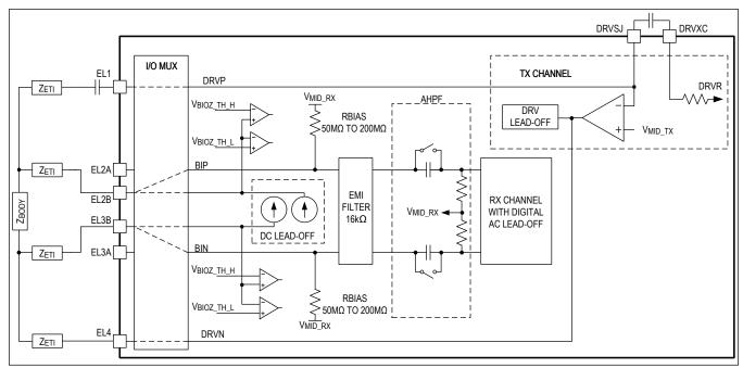
Figure 15. BioZ DC Lead-Off Detection with Internal Sense
