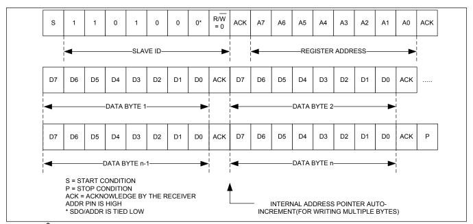
Figure 26. I<sup>2</sup>C Multibyte Write Transaction
