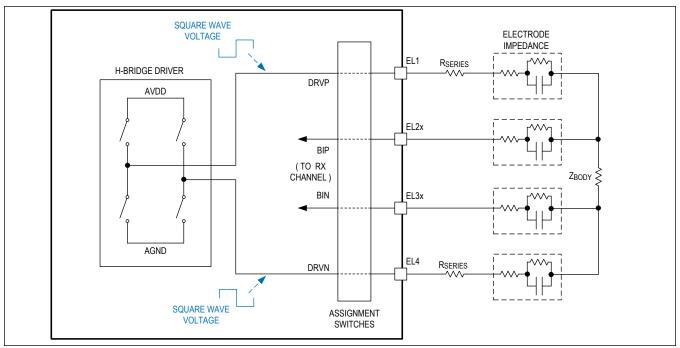
Figure 9. Bioimpedance Stimulus Generator — H-Bridge Square-Wave Voltage Mode
