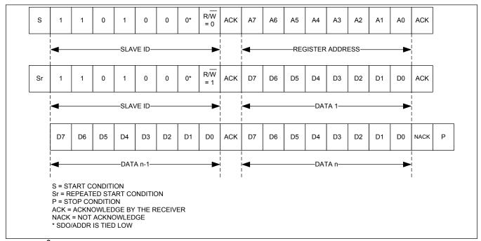
Figure 28. I<sup>2</sup>C Multibyte Read Transaction
