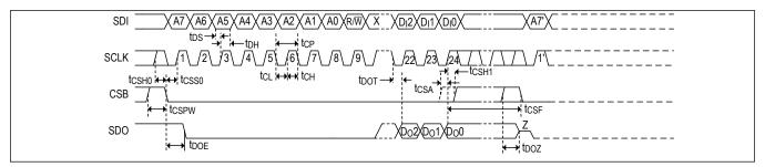
Figure 18. Detailed SPI Timing Diagram
