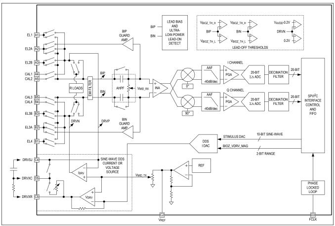
Figure 5. BioZ System Block Diagram
