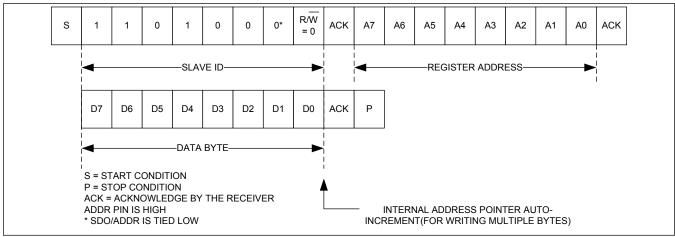
Figure 25. I<sup>2</sup>C Single-Byte Write Transaction
