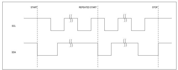
Figure 23. I<sup>2</sup>C START, STOP, and REPEATED START Conditions
