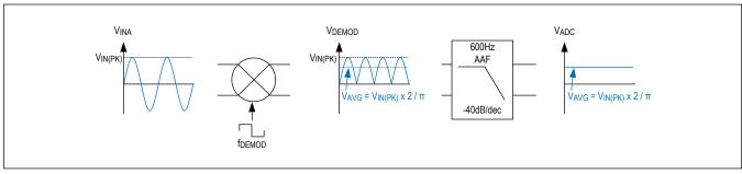
Figure 11. Square-Wave Demodulation for a Sine-Wave Stimulus (INA and PGA Gain Not Shown)
