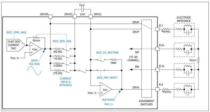
Figure 8. Bioimpedance Stimulus Generator — Sine-Wave Voltage Mode
