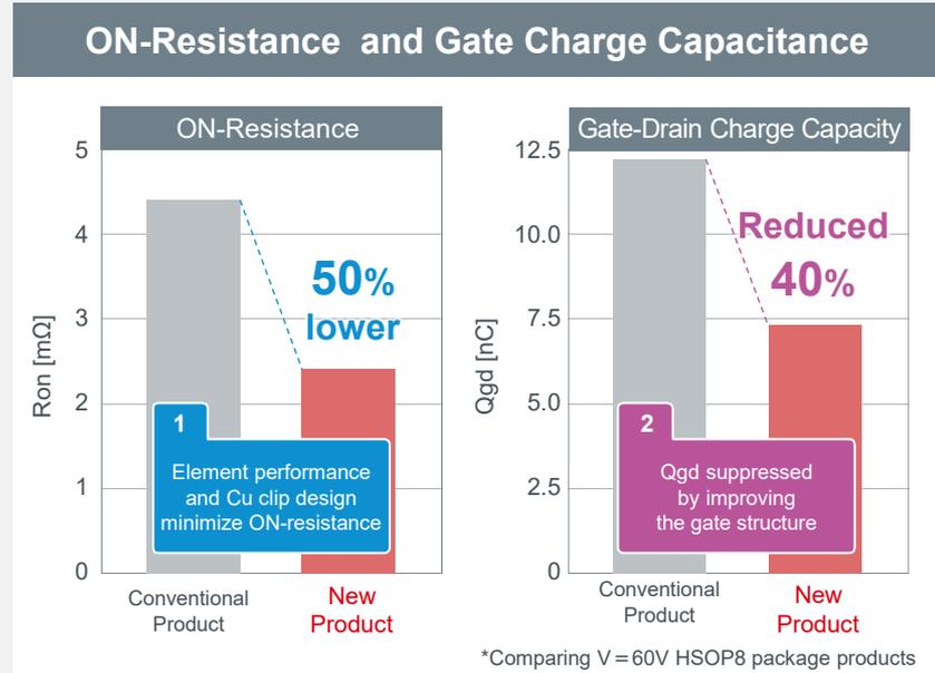
**Simultaneously improves gate charge capacitance, which has a trade-off relationship with ON-resistance**
